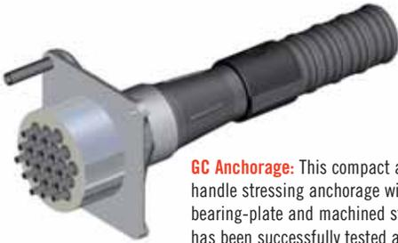
**GC Anchorage:** This compact and easy to handle stressing anchorage with a cast iron bearing-plate and machined steel anchor-head has been successfully tested and confirmed for cryogenic applications. The GC Anchorage, VSL's new generation of anchorage, replaces the extensively used EC Anchorage.
