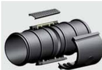
In addition to the standard steel spiral ducting, VSL offers the **PT-PLUS®** high resistance plastic duct with improved corrosion protection and also better force distribution along the tendon's length as a result of the reduced friction coefficient.
