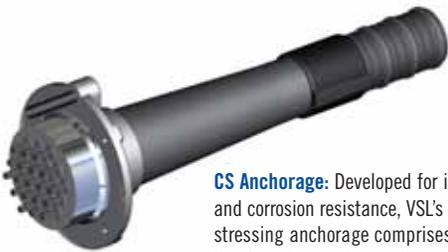
**CS Anchorage:** Developed for increased fatigue and corrosion resistance, VSL's high performance stressing anchorage comprises of a cast iron bearing-plate and a machined steel anchor head. The anchorage can be supplied with full encapsulation if greater corrosion protection is required.
