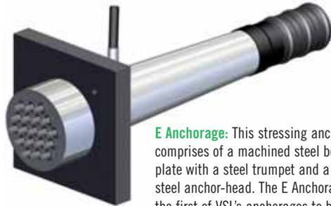
**E Anchorage:** This stressing anchorage comprises of a machined steel bearing-plate with a steel trumpet and a machined steel anchor-head. The E Anchorage was the first of VSL's anchorages to be confirmed for cryogenic applications.
